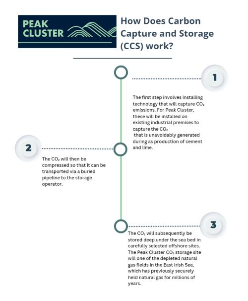
CCS is a mature technology that can capture up to 95% of CO<sub>2</sub> emissions produced in industrial processes. We will capture CO<sub>2</sub> on site from existing cement and lime plants in the Peak District and other industry sites along the pipeline route.
